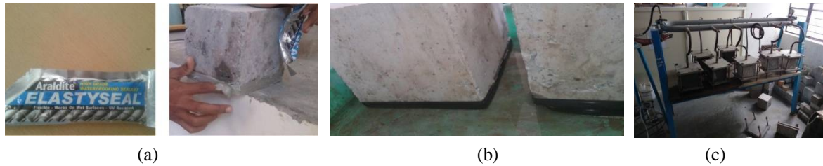
Fig.6- (a) Preparation of concrete cubes for sorptivity test (b) Concrete specimens kept in 5mm of water level for Sorptivity test (c) Permeability test setup.
