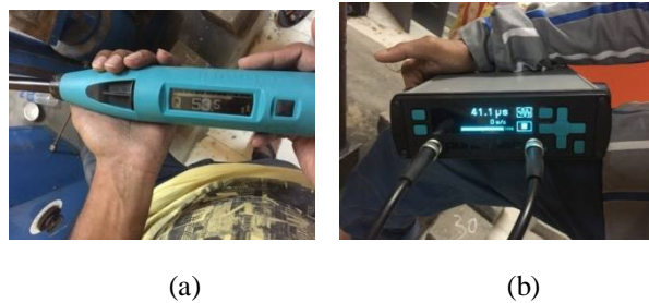
Fig.4- (a) Rebound hammer (b) Ultra sonic pulse velocity.
